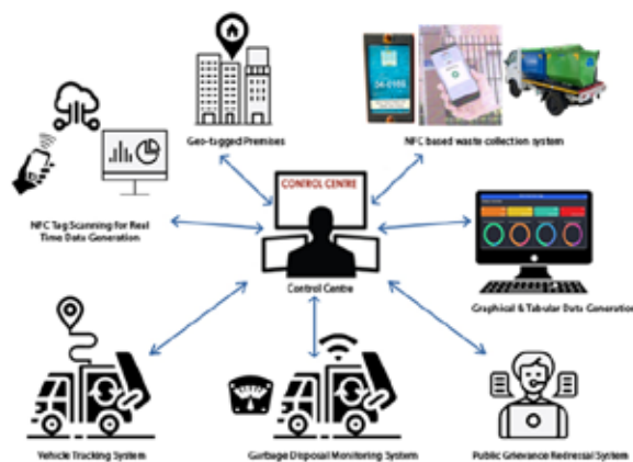
Figure 6: Features of the NFC based smart solid waste management system Source: Authors
